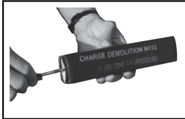
Figure 14-9. Priming of C4 demolition blocks with MDI.
