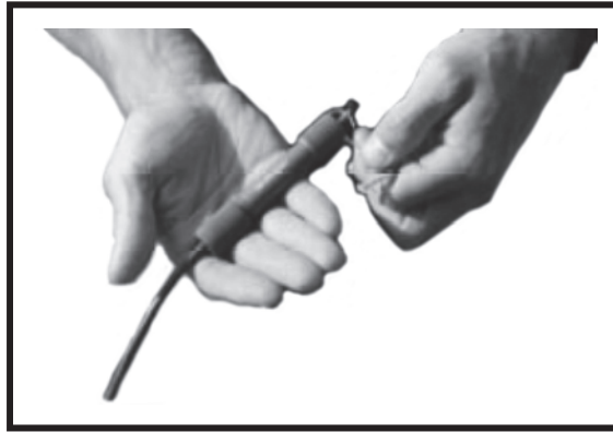
Figure 14-15. M81 fuse igniter with the M14 time fuse delay.
