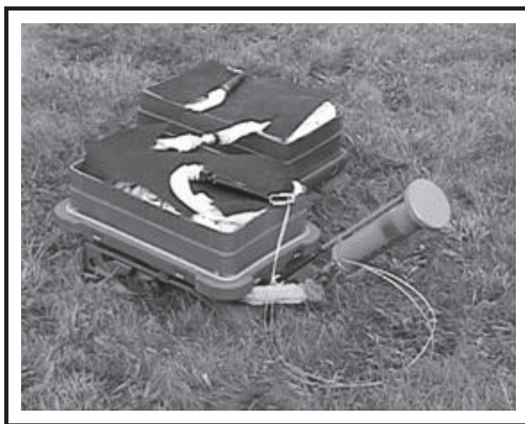
Figure 14-22. MK7 Antipersonnel Obstacle-Breaching System (APOBS).
